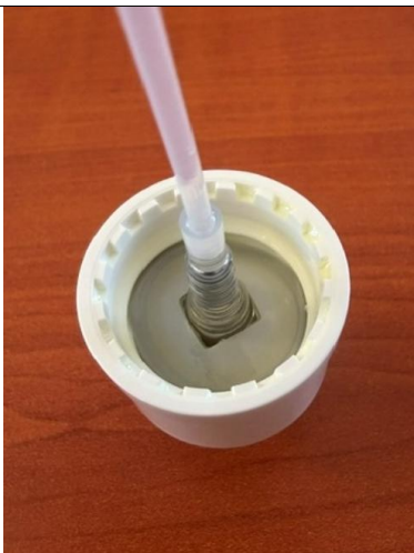
Figure 2. Inside of the spray closure showing the EPE foam sealing disc at the neck-sealing interface.
