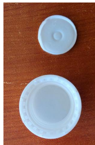
Inside of the closure showing the sealing EPE foam interface.
